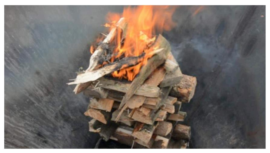
let the fire burning to about 1/3 from the top of the stack or pyramid creating a strong up-draft which pulls in air at the side walls of the pit. Spread then the feedstock at the bottom.
