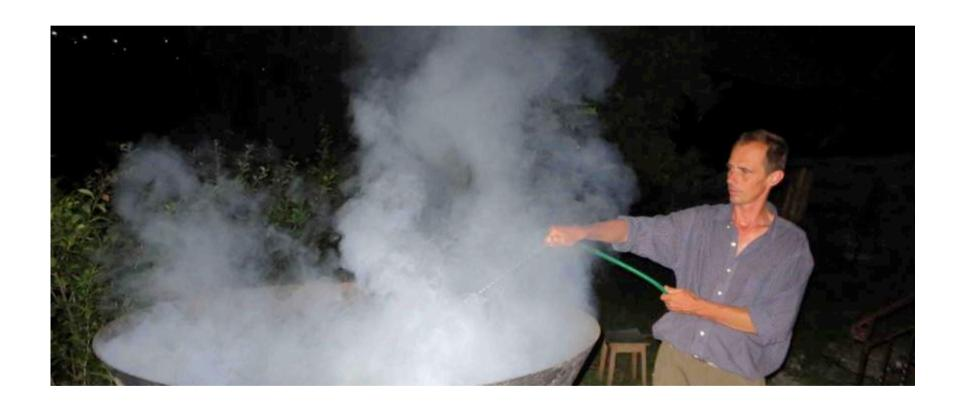
Quench the kiln with water partially activates the biochar (cleaning of the biochar pore structure and increasing surfaces)
